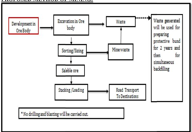
Opencast semi mechanized method of mining will be done.
